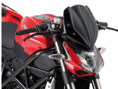
247N Universal screen for naked bikes, black colour (W x H) 29 cm x 28,5 cm The inside is painted in matt colour to prevent the front light from reflecting
